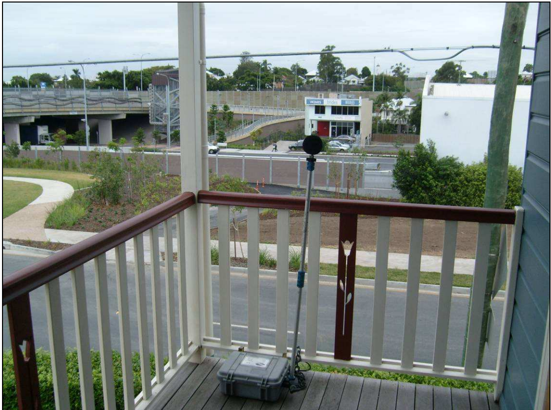
Photo A2: ML2 – Noise logger at 6 Albert Street, Woolloongabba, with a view to Ipswich Road and the Clem7 tunnel entrance at the top left.
